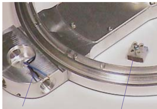
Motor pigtail Terminal block(removed)
